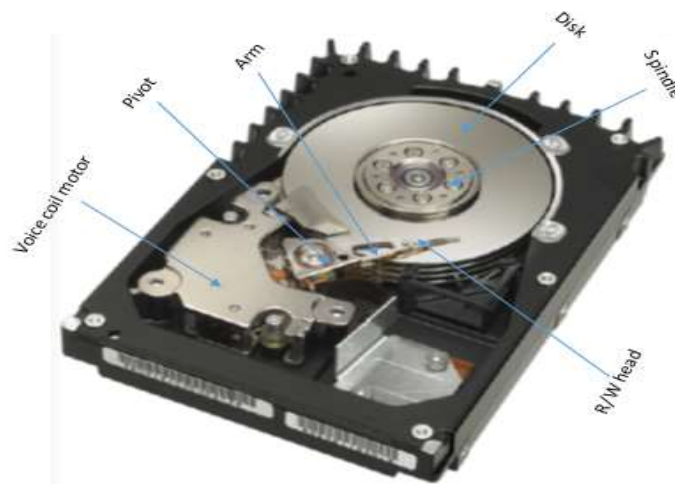
Fig.1: A typical hard disk drive servo system
